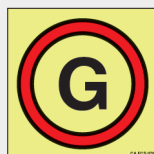
EMERGENCY GENERATOR CA FCS 076 C
