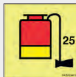
PORTABLE FOAM APPLICATOR UNIT OR RELEVANT SPARE TANKS
