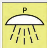
SPACE OR GROUP OF SPACES PROTECTED BY POWDER FIRE EXTINGUISHING SYSTEM
