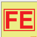
LOCKER WITH FIREMAN'S OUTFIT CA FCS 067 C
