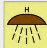
SPACE OR GROUP OF SPACES PROTECTED BY GAS OTHER THAN CO 2 FIRE EXTINGUISHING SYSTEM
