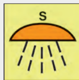
SPACE OR GROUP OF SPACES PROTECTED BY SPRINKLER OR HIGH PRESSURE WATER FIRE EXTINGUISHING SYSTEM
