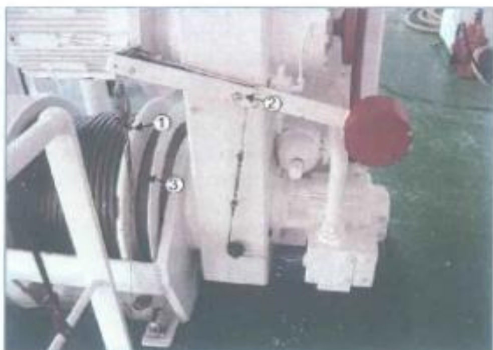
Fig. 2 Arrangement for brake remote release cable
