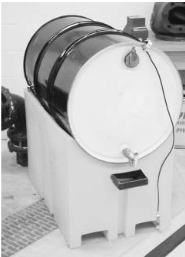
FIGURE 3.2 Typical flammable-liquids transferring arrangement
